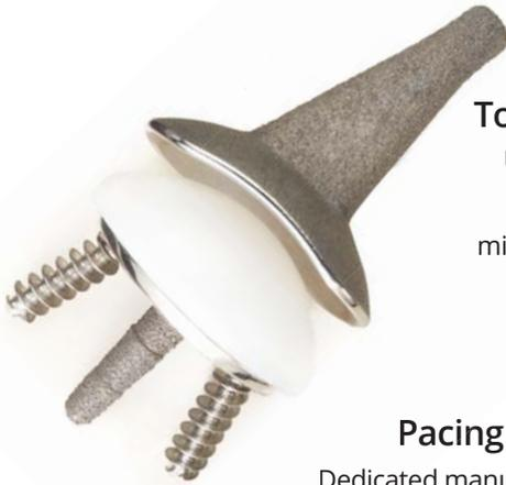
**Total joint implant** – UHMW polyethylene and cobalt chrome; 5-axis milling, EDM, Swiss turning, and hand polishing.
