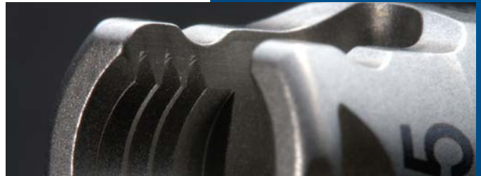
Polyaxial spinal screw – Head on 13-axis lathe; screw on a Swiss lathe with thread whirling.
